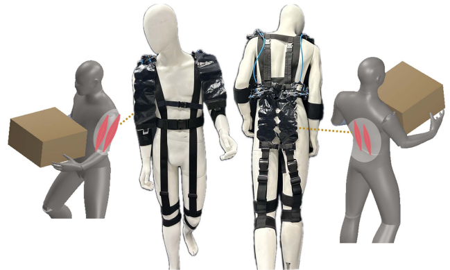
Fig. 1. Integrated assistive suit equipped with FIAMs. Two parallel artificial muscles are connected to the back, and another two are connected to the upper arm, respectively. This suit is designed to support general lifting motions, primarily utilizing the muscles of the back and upper arms.
